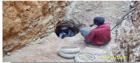
Photo 1: Natives taking alluvial ore from pit of about 6m to pan for Gold (Goni area).
